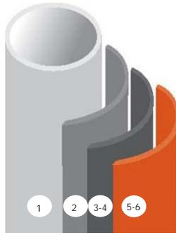
**1 SHOT-BLASTING TO WHITE METAL** First, all of our metal is cleaned to white metal. We strip it to its purest form using our state-of-the-art shot-blast system. This process removes all the impurities from the metal, especially at the weld joints. It's more effective than traditional acid cleaning and also creates a more textured surface, allowing for better adhesion of the Powder-coat.
